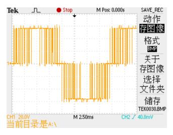
The output PWM waves of the cell
