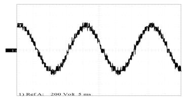
The line voltage wave of 5cells in series
