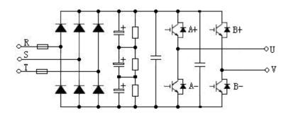
The power cell structure of two-quadrant high voltage inverter
