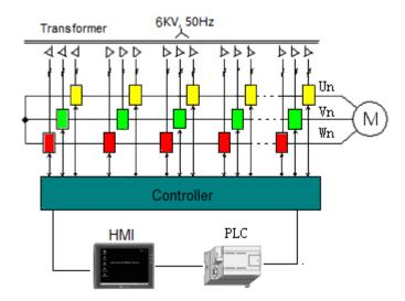
The structure of high voltage inverter
