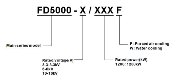
For example: FD5000-6/2200F, the inverter rated votage is 6kV, and rated output power is 2000kW, forced air cooling.
