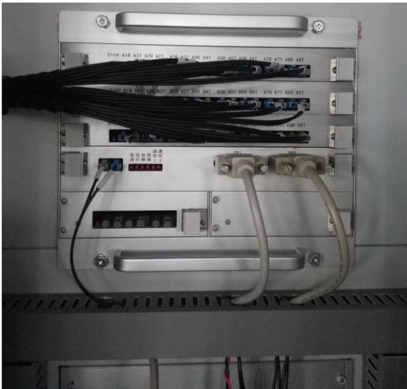
There are four types basic circuit board: motherboard, main control board, signal conversion board, fiber board.
